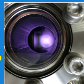
Energetic 3" diameter plasma at 200 Torrs 6KW
